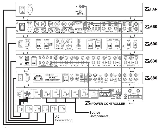
**<sup>★</sup>** Disable Current Sense via front panel Dip Switches
