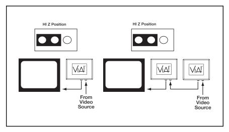
For applications where different, independent video is displayed on each VIA!/TV, run separate feeds of RG-6 or RG-59 from a video switcher (ELAN Z•880 or S12) to each VIA!/TV as shown below. Keep the 75 Ohm Termination Jumper in the **75 Ohm** position.
