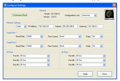
7. Confirm the unit shows up in the GC-100 Discovery and Configuration Utility with the new IP address.
