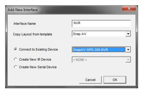
3. Finally, add the source to the desired zone controller input as normal and arrange the appropriate selections to manage your Display source to select the SnapAV NVR monitor out for one-way control from the g! Viewer.
