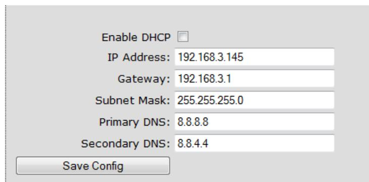
The image shows a configuration form for static IP settings. It includes a checkbox for "Enable DHCP" which is unchecked. Below it are five input fields: "IP Address" with the value "192.168.3.145", "Gateway" with "192.168.3.1", "Subnet Mask" with "255.255.255.0", "Primary DNS" with "8.8.8.8", and "Secondary DNS" with "8.8.4.4". At the bottom of the form is a "Save Config" button.
