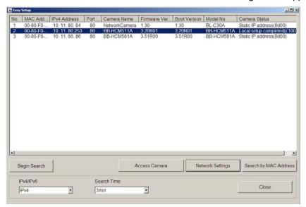
4. Select the desired camera, and then click the **Access Camera** button. After a short delay you will see a new browser window with the initial password screen below:
