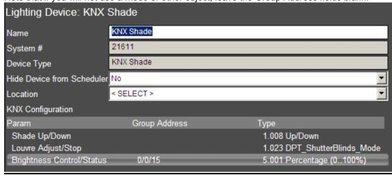
Lighting Device: KNX Shade KNX Shade Name 21611 System # KNX Shade Device Type Hide Device from Scheduler No. < SELECT > Location KNX Configuration Group Address Param Type Shade Up/Down 1.008 Up/Down 1.023 DPT ShutterBlinds Mode Louvre Adjust/Stop √ 5.001 Percentage (0..100%) 0/0/15 Brightness Control/Status 5.004 Percentage (0..255%)
