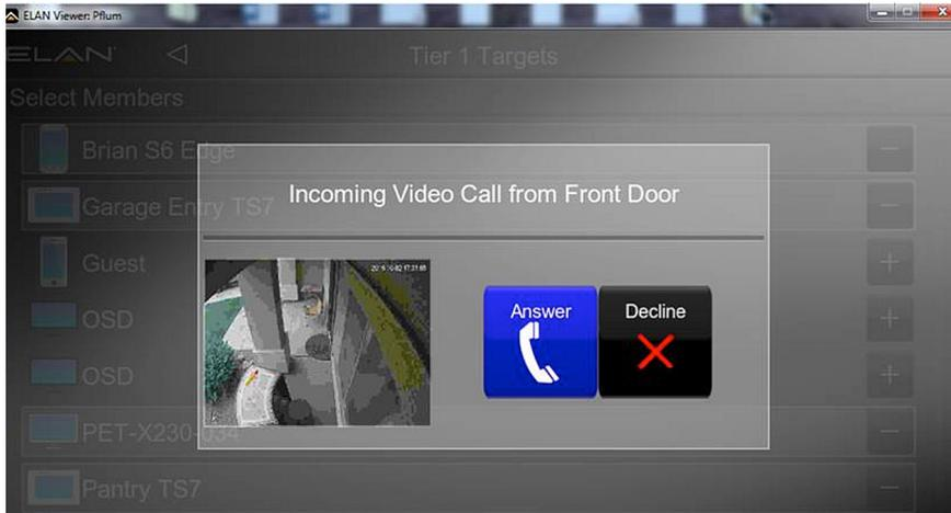
\*Doorstations with its camera added as a separate video device in Configurator and selected in the Video field in its doorstation settings rather than the default "Built In" setting, will allow ELAN to initiate the video stream before a SIP call is answered.
