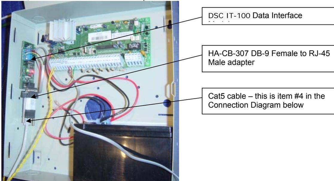
2. If you are using a hub enclosure, be sure to leave room for the cable and DB-9 to RJ-45 adapter to connect easily to the DSC IT-100.
